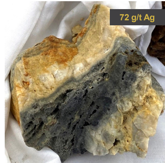
Low temp., high grade Ag "ribbon veins" that replace earlier formed skarn in the Barcelona Target
