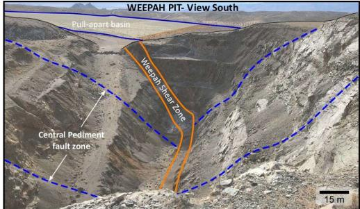
Historical open pit with view of Weepah shear zone and intersection of newly identified Central Pediment fault
