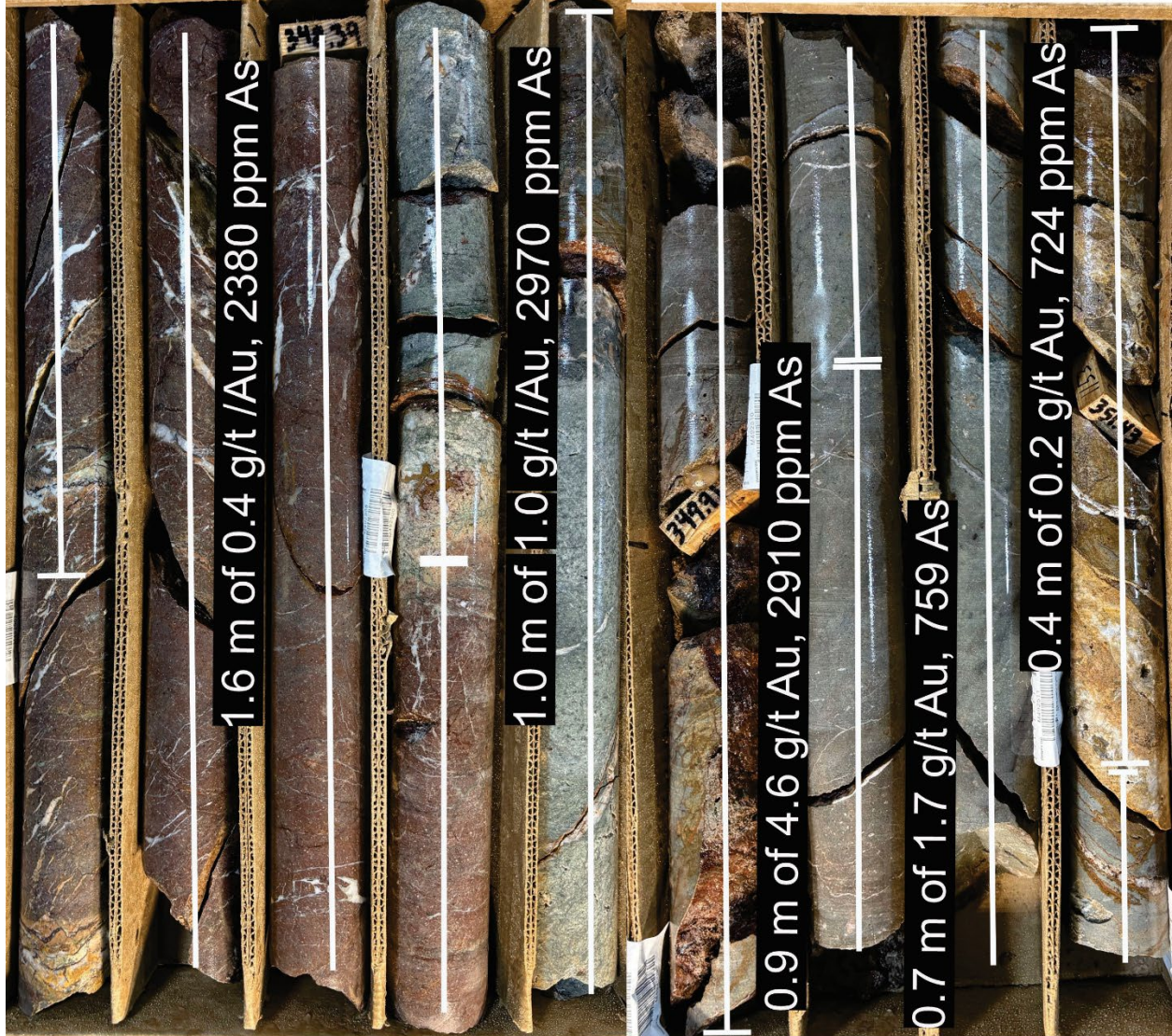
Figure 6. Gold and Arsenic-enriched drill core from HSC-002. The composite intercept is 4.6 m of 1.4 g/t gold and 2252 ppm arsenic starting at 347.1 meters hole depth.
